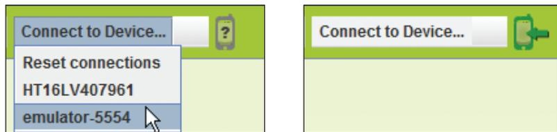
During the connection process the icon to the right of the “Connect to Device” button first changes to flashing yellow, but becomes solid green when the Emulator is connected. The application then gets loaded onto the screen and is ready to run.
