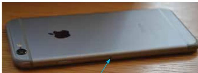
Push the SIM tool firmly into this hole to access the SIM tray and insert a SIM card (see pages 12-13 for details)
