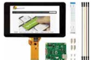
When you have gathered together all necessary components they can be connected as shown above – but the Raspberry Pi is not yet functional as the SD card doesn't contain an operating system.
