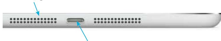
**Lightning Connector.** Connect the Lightning Connector here to charge the iPad, or connect it to another computer. (Some models of the iPad Pro – 2018 and later – use a USB-C Connector rather than a Lightning Connector. This means it can also be used with a USB-C flashdrive – see page 72 for details).
