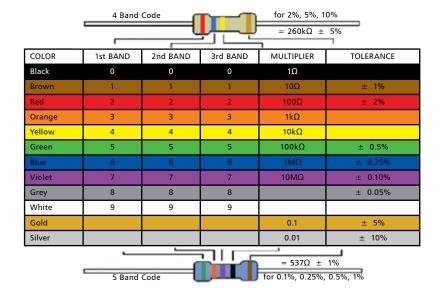
The four-band is the most common as it is used for wide tolerance (and hence cheaper) resistors found in many circuits. The five-band code is used where very accurate resistance values are needed.
