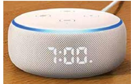
The services and information delivered through the Amazon Echo by Alexa are cloud-based, which means that all of the data is stored in an Amazon computer (server) and then delivered through the Amazon Echo when it is requested. Nothing is physically stored on the Echo – it is merely a delivery system. The Echo works through connecting to your home Wi-Fi network: without Wi-Fi it will not function properly.
