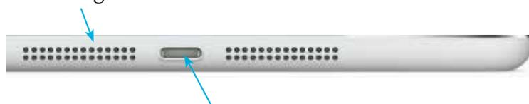
**Lightning Connector.** Connect the Lightning Connector here to charge the iPad, or connect it to another computer. Some models of the iPad Pro (2018 and later) and the iPad Air (4th generation) use a USB-C Connector rather than a Lightning Connector. This means it can also be used with a USB-C flashdrive – see page 70 for details.
