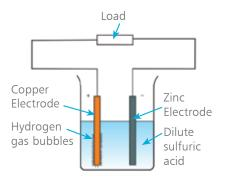
The sulfuric acid is poured into a container, and the electrodes are placed into the electrolyte. If the two electrodes are then connected together outside of the cell, a current will
