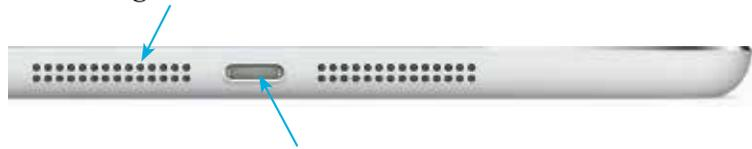
**Lightning Connector.** Connect the Lightning Connector here to charge the iPad, or connect it to another computer. Some iPad models have a USB-C Connector, rather than a Lightning Connector. These include: iPad Pro 11-inch (2nd generation and later), iPad Pro 12.9-inch (3rd generation and later), iPad Air (4th generation and later), and iPad mini (6th generation and later).
