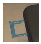
Insert the SIM card into the SIM tray and return it into the slot in the phone. (Some SIM trays have compartments for different sizes of SIM cards)
